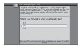
4. Highlight the channel you have to tune your TV to see cable box programming, and press OK (a screen appears reminding you to connect your G-LINK cable to your TV and cable box).
