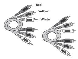
Use one set of composite audio/video cables to connect to the TV's input; another set to connect to the TV's output.
